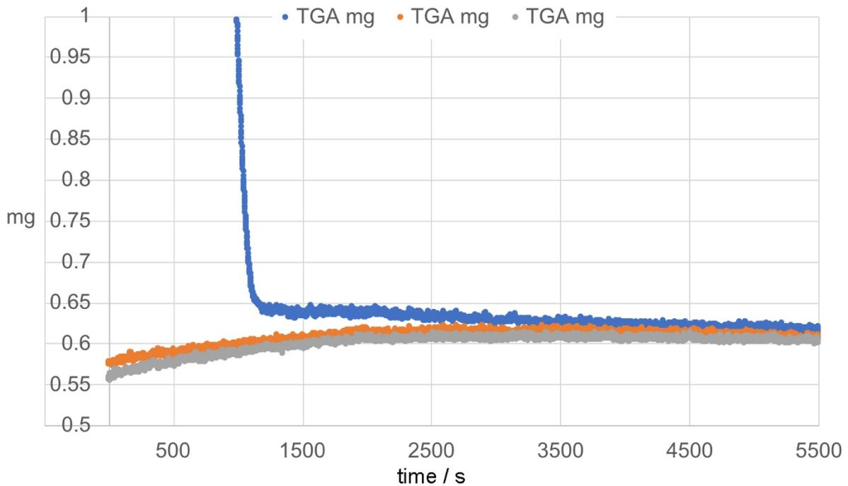
Figure 4: Thermogravimetric Analysis (TGA) of DT 6060 on steel. Three consecutive runs with the same coating were performed per the temperature profile shown in Figure
