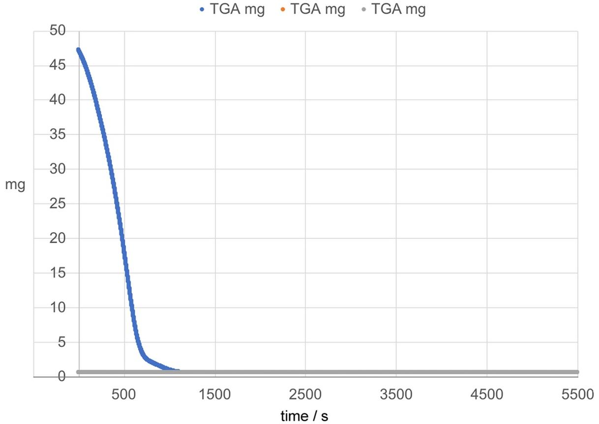
Figure 2: Thermogravimetric Analysis (TGA) of DT 6060 on steel. Three consecutive runs with the same coating were performed per the temperature profile shown in Figure 1.
