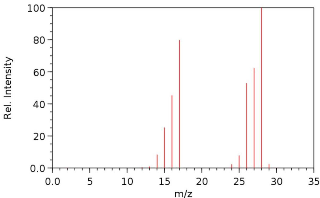
Figure 6: Mass spectrum of the gas phase above DT-420 (run 2, 3500 s). The mass spectrum is consistent with a mixture of ethylene (and potentially other hydrocarbons) and ammonia (reference: <https://webbook.nist.gov/chemistry>).
