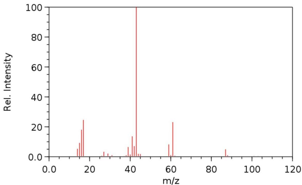
Figure 5: Mass spectrum of the gas phase above DT-420 (run 1, 1500 s). The mass spectrum is consistent with a mixture of isopropyl acetate and ammonia (cluster at masses 17, 16, 15 and 14). (reference: <https://webbook.nist.gov/chemistry>).
