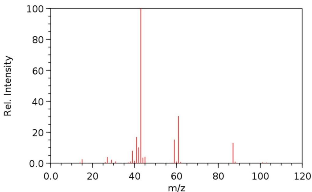
Figure 4: Mass spectrum of the gas phase above DT-420 (run 1, 1000 s). The mass spectrum is consistent with a mixture of isopropyl acetate and aliphatic hydrocarbons (reference: <https://webbook.nist.gov/chemistry>).
