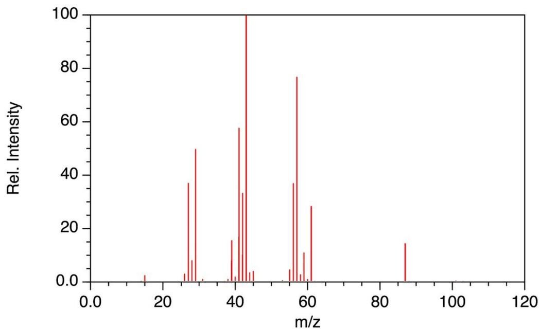
Figure 3: Mass spectrum of the gas phase above DT-420 (run 1, 500 s). The mass spectrum is consistent with a mixture of isopropyl acetate and aliphatic hydrocarbons (reference: <https://webbook.nist.gov/chemistry>).
