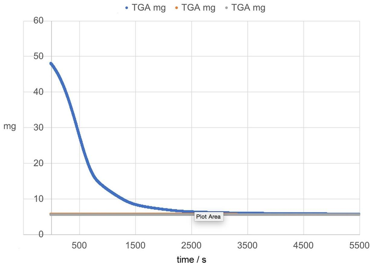
Figure 2: Thermogravimetric Analysis (TGA) of DT-420 on steel. Three consecutive runs (blue: first run; orange: second run; gray: third run) with the same coating were performed according to the temperature profile shown in Figure 1.
