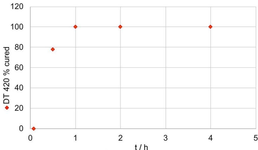
Figure 5: Thermal Curing of DT-420 on Q-panels
