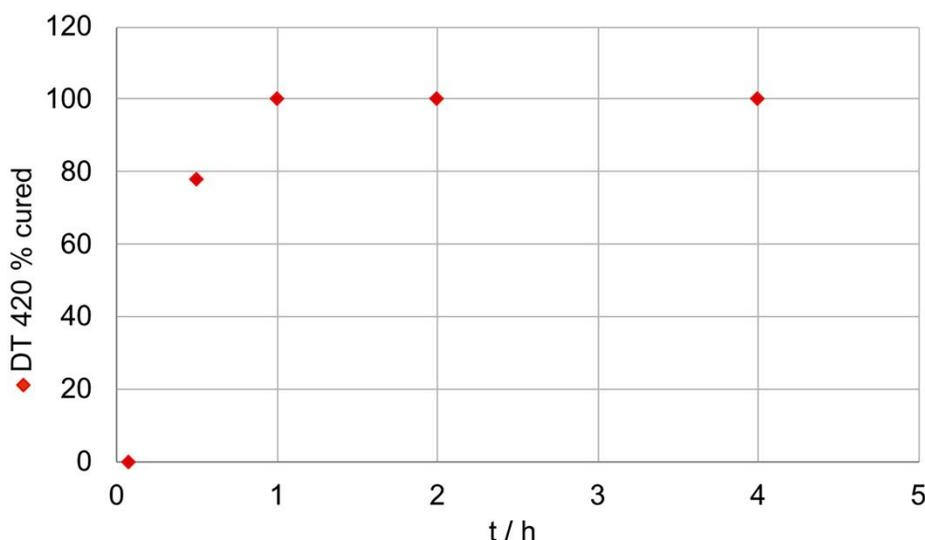
Figure 3: Thermal Curing on Aluminum. DT-420 is completely cured after 1 h at 120 °C/250 °F regardless of the film thickness.
