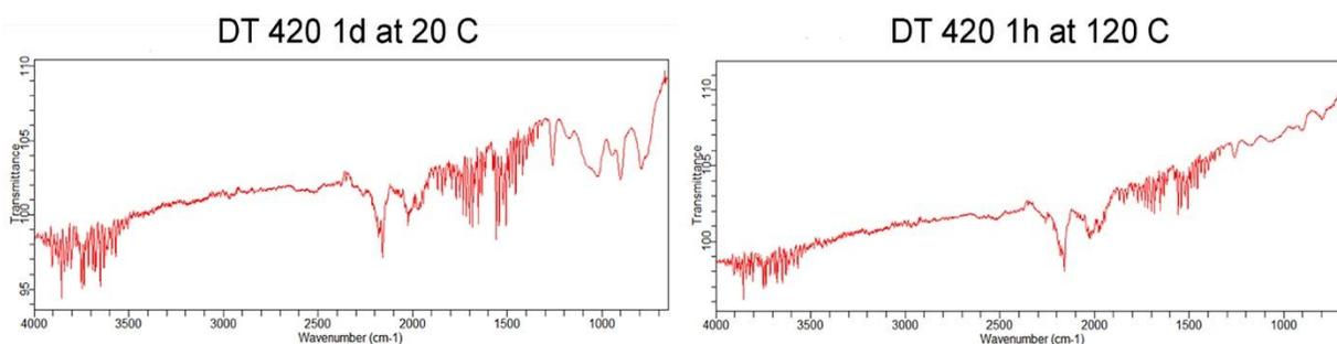
Figure 2: FTIR spectra of DT-420 on aluminum. Left: 24 h at  $20\text{ }^\circ\text{C}$  /  $70\text{ }^\circ\text{F}$ , film thickness of 5 microns. Right: thermal curing, 1 h at  $120\text{ }^\circ\text{C}$  /  $250\text{ }^\circ\text{F}$ , film thickness of 4 microns.
