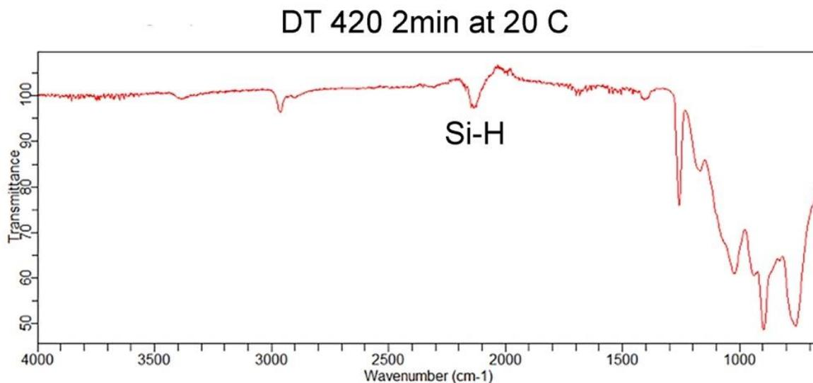
Figure 1: FTIR spectrum of DT-420 coated aluminum surface at 5 minutes after coating. Estimated film thickness is 10 microns.
