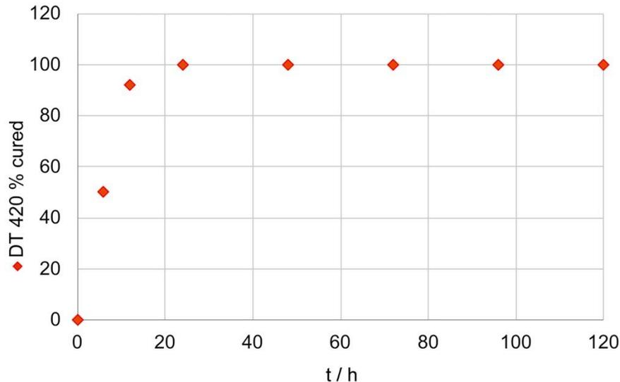
Figure 6: Ambient Curing of DT-420 on Q-panels
