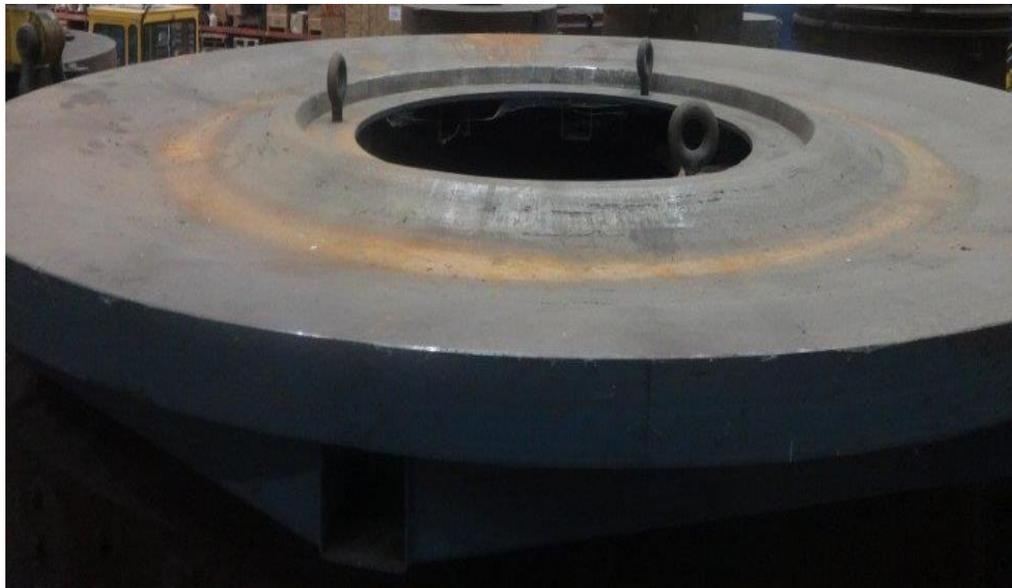
**SOLUTION:** Dyna-Tek’s mold sealer and release coating system. The Staging/Resting Plate was lightly mechanically etched so as to remove impurities, and clean the metal surface. Upon completion of this step, the surface was cleaned with an approved solvent so as to remove any remaining impurities.
