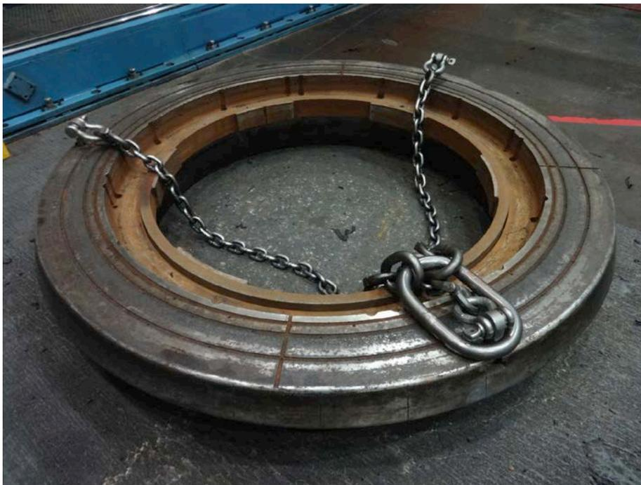
**SOLUTION:** Dyna-Tek's mold sealer and release coating system. The bladder ring was lightly mechanically etched so as to remove impurities, and clean the metal surface. Upon completion of this step, the surface was cleaned with an approved solvent so as to remove any remaining impurities.
